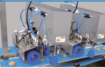
The Secondary forming option on the forming conveyor shapes the products consistently.
