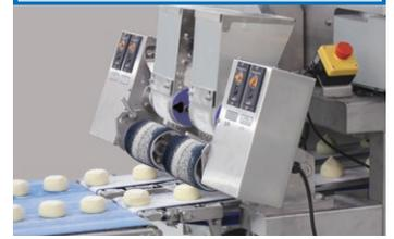
Presses down the top of the product using the press roller with flour duster.
