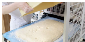
Place the dough on the conveyor from a tray. Then all you have to do is enter the cutting and weight and push the start button.
