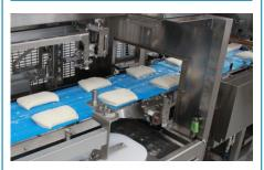
When dividing different shape bread doughs from the VX222 you can use "Bypass Mode" on the Punch Rounder which acts as a conveyor without rounding mechanism engaged, for quick changeovers for making a variety of breads.
